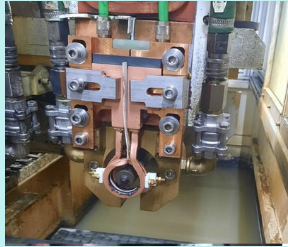
Figure 10. As scheduled preventive maintenance, replaced the induction quench ring and coil, and a new set was installed to maintain desirable hardness and microstructure.
