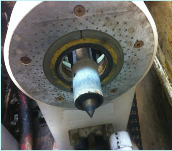
Figure 9. Induction quench ring and coil. Debris plugging quench holes will result in low hardness and undesirable microstructure.
