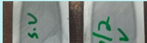
Figure 6. Acceptable Induction hardening pattern.
